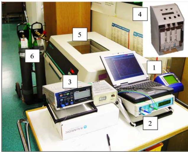
Fig. 1 The experimental setup for the in vitro pO_2 study showing the NV (1) and LX (2) monitors collecting the data from oxygen sensors. Two temperature probes (3) measured the temperature in the equilibrator (4), which was inserted in the warming box (5) and bubbled with high precision O_2 gases (6)
